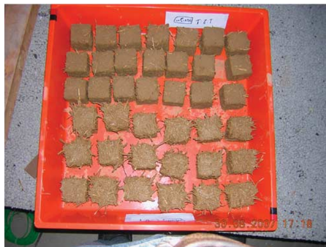
Figure 1: Samples prepared for drying test and water absorption.
